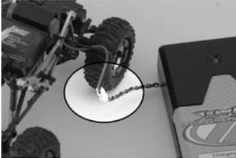
3. Plug the battery lead into the charger lead. The RED LED will light up and stay solid while charging. When the battery is fully charged the light will shut off (approximately 20 minutes). If the charger light only lights up for about a minute, the AA batteries inside the charger are low and should be replaced.
