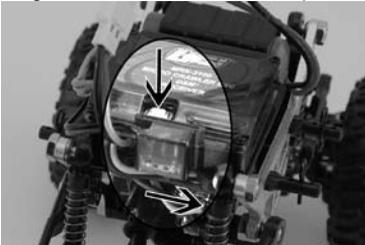
5. While pressing the white "Bind" button, slide the switch to the "On" position. When the green LED begins to flash rapidly release the bind button.
