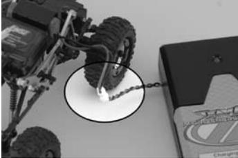
3. Plug the battery lead into the charger lead. The RED LED on the charger will light up and stay solid while charging. When the battery is fully charged the light will shut off (approximately 20 minutes). If the charger light only lights up for about a minute, the AA batteries inside the charger are low and should be replaced.
