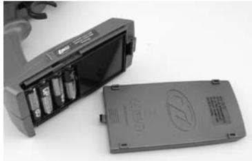
4. Remove the transmitter battery cover by sliding it in the direction noted on the cover. Install four (4) AA batteries into the battery holder. Pay close attention to the correct direction of the positive (+) and negative (-) ends as marked. Once all 4 batteries have been installed, reinstall the battery cover.
