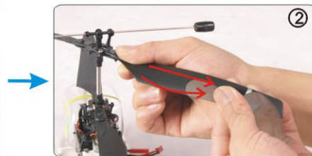
(2) 主旋翼攻角调整方法 Adjustment way to angle of attack of main blades.
