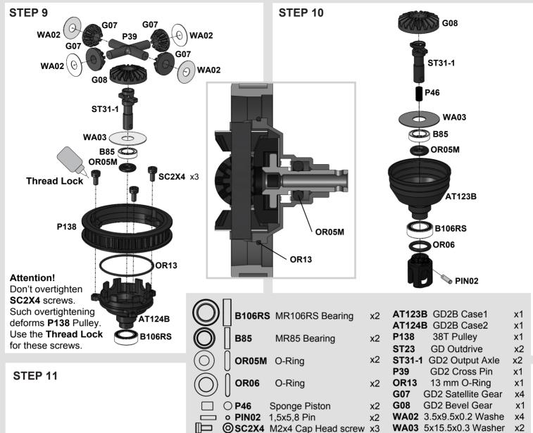
Fill with desirable silicone oil (not included). Screw AT123B GD2B Case with 10mm wrench slowly. The excessive oil will go out through the ST31-1 axial hole.
