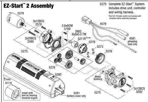
\*Part 5211R (roller clutch) not included with complete starter assembly packages.
