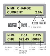
This program simply charges the battery using the current you set. The charge current ranges from 0.1 to 5.0A.
