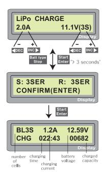
The value on the left side of second line sets a charge current and the value on the right side of second line sets the voltage of the battery pack.
