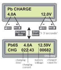
Set up the charge current on the left and the nominal voltage of the battery on the right. The charge current ranges from 0.1 to 5.0A and the voltage should match with the battery being charged.
